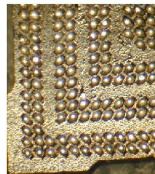
Grypper G40 test socket assembly: solder balls attached
